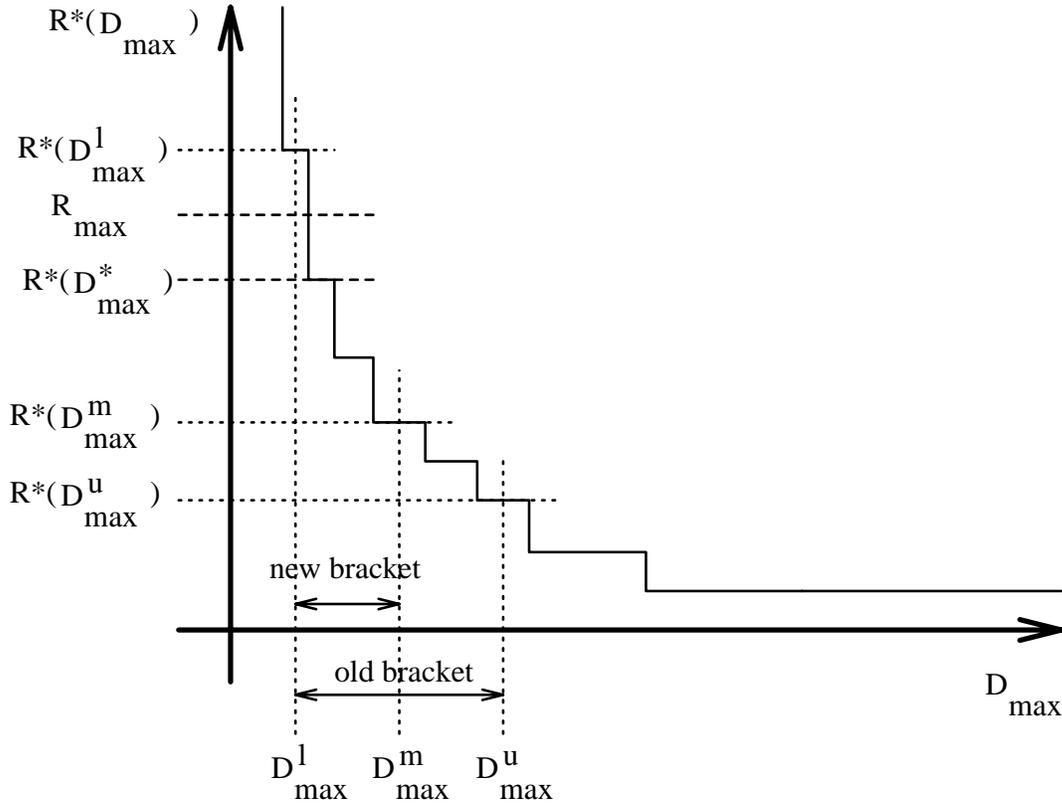
Fig. 1. The  $R^*(D_{max})$  function, which is a non-increasing function exhibiting a staircase characteristic. The selected  $R_{max}$  falls onto a discontinuity and therefore the optimal solution is of the form  $R^*(D_{max}^*) < R_{max}$ , instead of  $R^*(D_{max}^*) = R_{max}$ .
