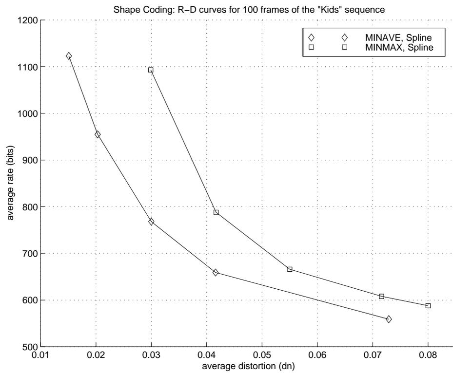
Fig. 17. Rate-distortion performance of MINAVE and MINMAX algorithms.
