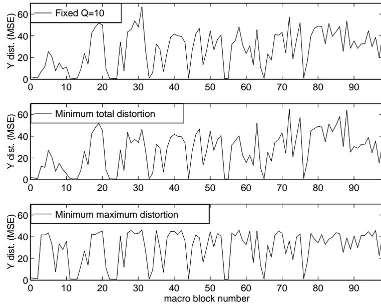
Fig. 3. MSE of each macro block of the luminance channel; First row: MSE for a fixed quantizer step size of  $Q=10$ . Second row: MSE for the minimum total distortion approach. Third row: MSE for the minimum maximum distortion approach.
