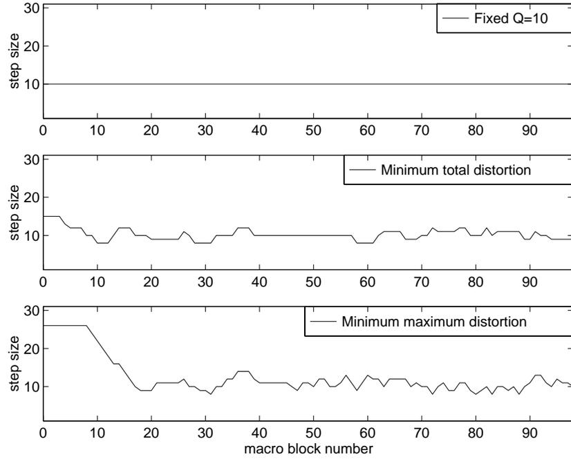
Fig. 2. Macro block quantizer step sizes; First row: fixed quantizer step size of  $Q=10$ . Second row: step sizes for the minimum total distortion approach. Third row: step sizes for the minimum maximum distortion approach.
