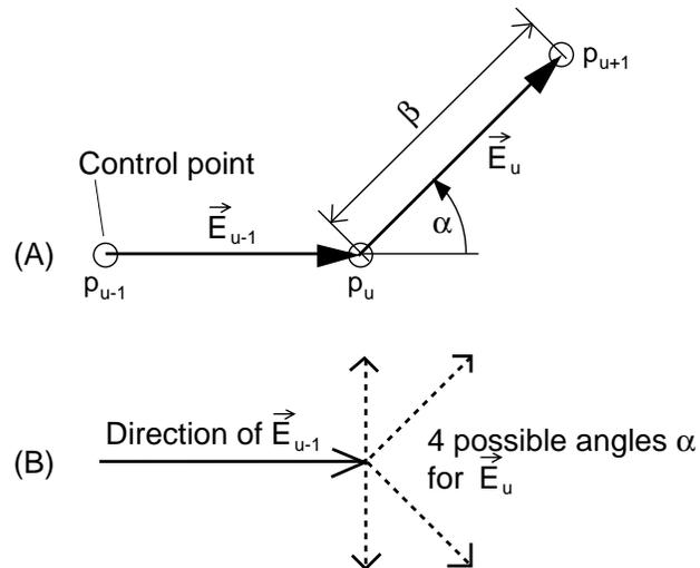
Fig. 16. Encoding of a spline control point.
