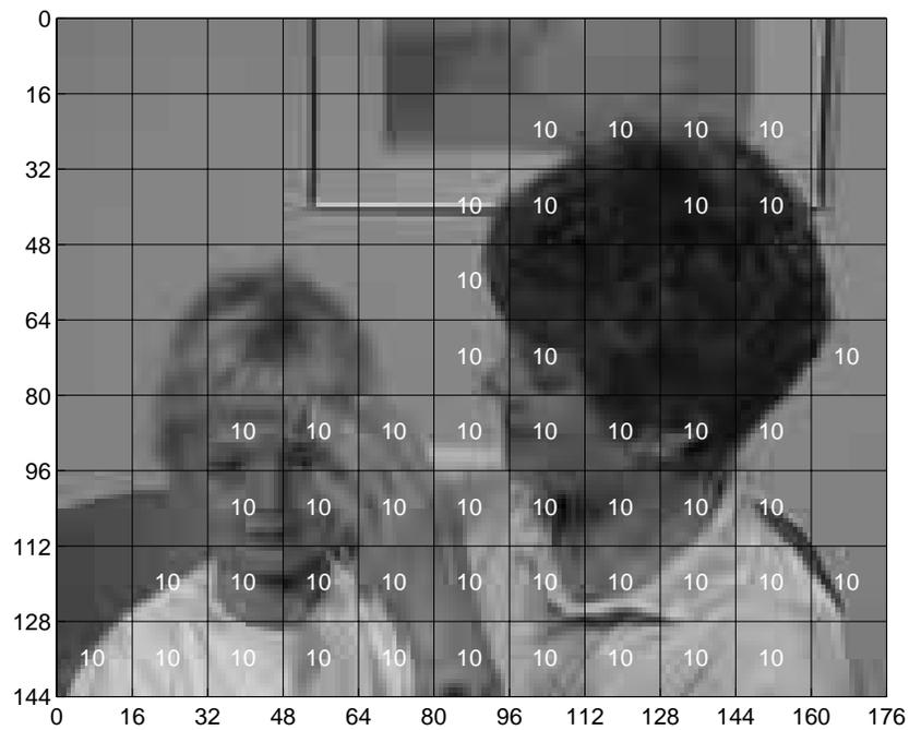
Fig. 8. Quantizers in the fixed quantizer scheme.
