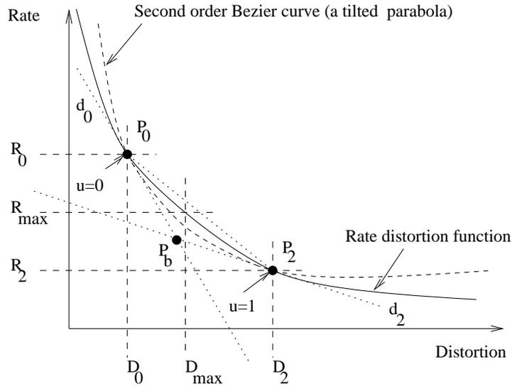
Figure 7: Continuous rate distortion curve and the second order Bezier approximation between two bracketing points.
