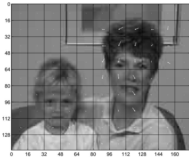
Figure 14: The predicted frame and the DVF for TMN4 block matching.
