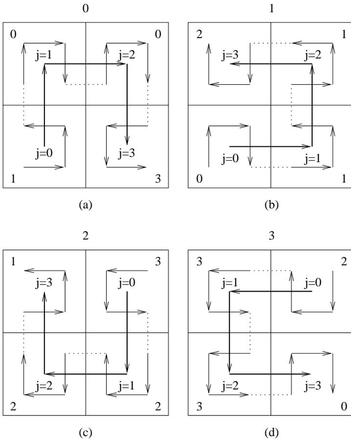
Figure 5: The four possible first order Hilbert curves (-) with the respective second order Hilbert curves underneath (-). The orientations  $O_{l,i}$  are shown on top of the squares and the orientations  $O_{l-1,4*i+j}$  are shown in the corners of the smaller squares.
