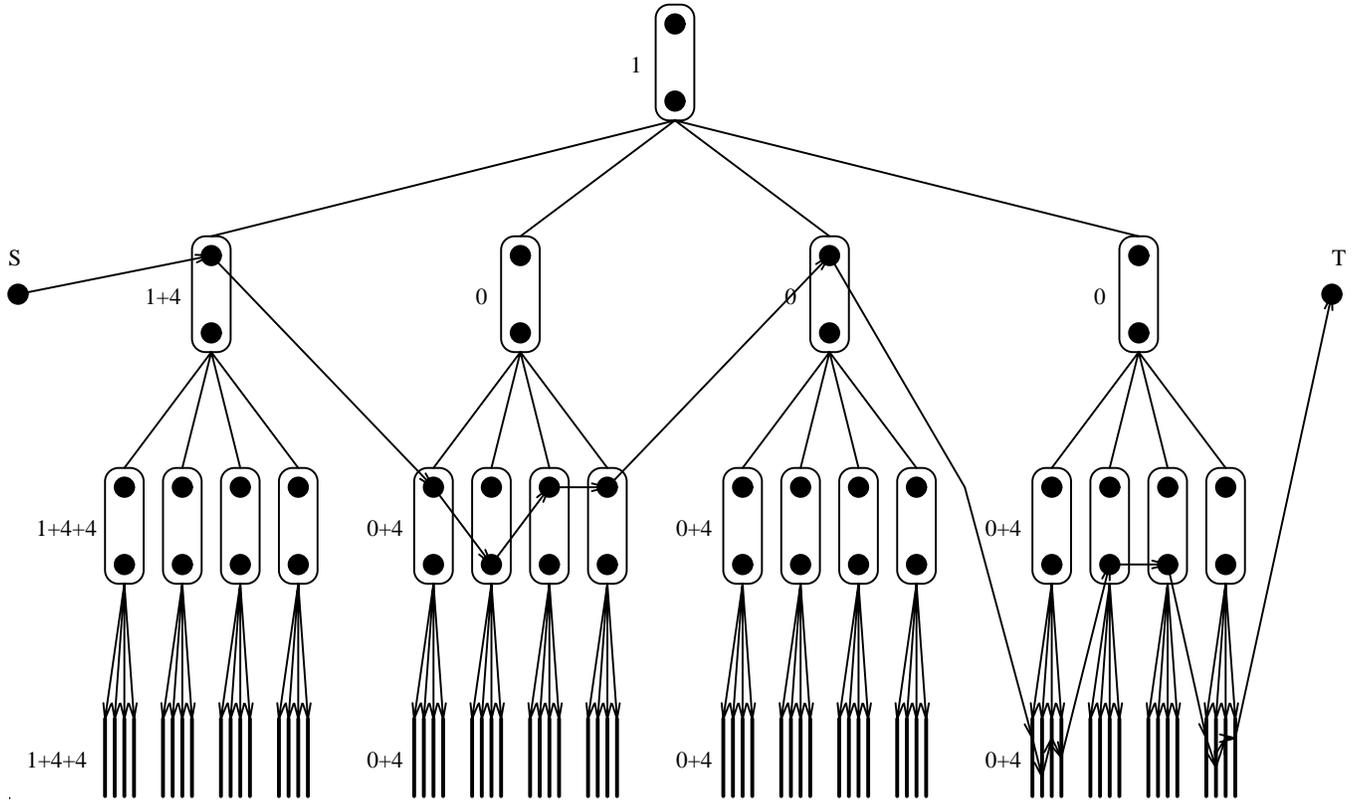
Figure 10: The recursive distribution of the quad-tree encoding cost among the trellis nodes for a quad-tree of depth 4 and an optimal path.
