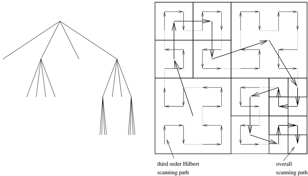
Figure 11: Quad-tree decomposition corresponding to the optimal state sequence. The left figure shows the graphical representation of the QT which corresponds to the frame decomposition in the right figure. The right figure shows the level  $n_0$  scanning path, which is a third order Hilbert curve, and the resulting overall scanning path.
