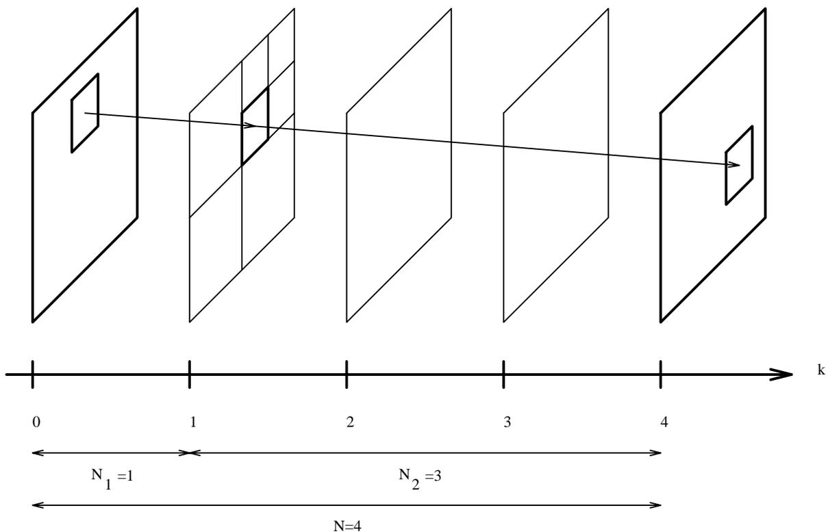
Figure 12: Motion compensated interpolation of the first frame using the two transmitted frames, which are the left most and the right most frame.
