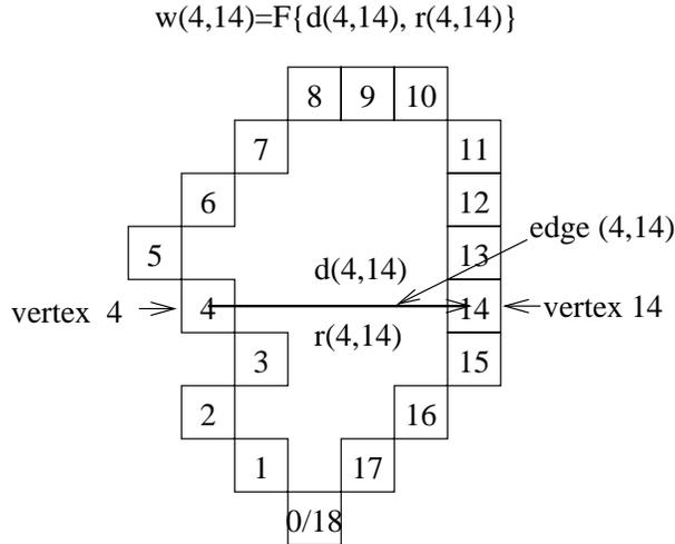
Figure 9: Each edge has a segment rate and a segment distortion associated with it. The edge weight is then a function ( $F\{\cdot\}$ ) of these rates and distortion. For class one distortion measures, this function is different than for class two distortion measures.
