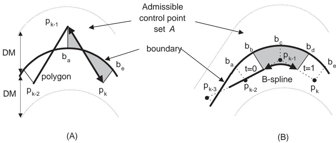
Figure 4: The definition of a state for a polygon and a second order B-spline curve. Figure (a) shows that for a polygon, knowing  $p_{k-1}$  makes the search for future control points independent from the control points already selected. Figure (b) shows that for a second order B-spline, knowing  $p_{k-2}$  and  $p_{k-1}$  makes the search for future control points independent from the control points already selected.
