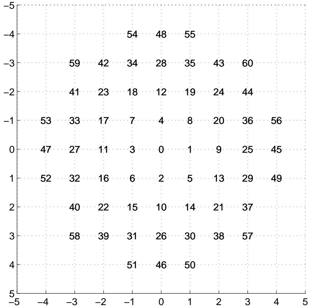
Figure 2: Vector increments for the definition and ordering of the admissible control point set. Note that vector  $v_j$  starts at 0 and ends at  $j$ .
