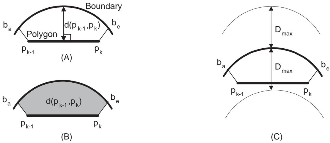
Figure 6: Three different ways for defining the segment distortion for a polygon-based approximation of the original boundary. Figure (a) shows the maximum distance, Figure (b) the error area, and Figure (c) the maximum distance band concept.
