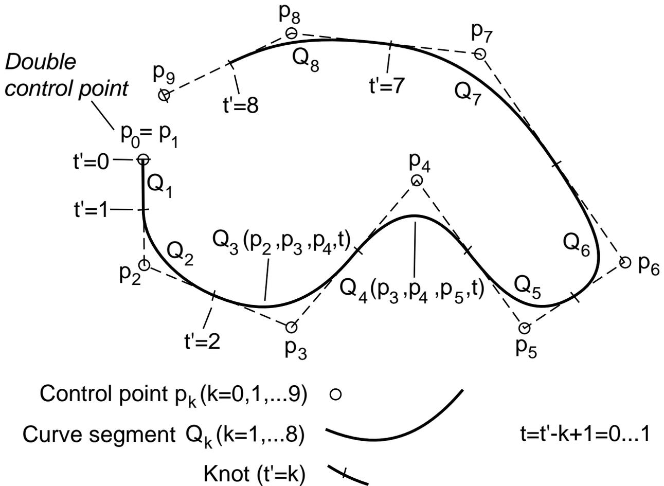
Figure 5: A second degree B-spline curve with 8 curve segments  $Q_k$  and a double control point at the beginning of the curve.
