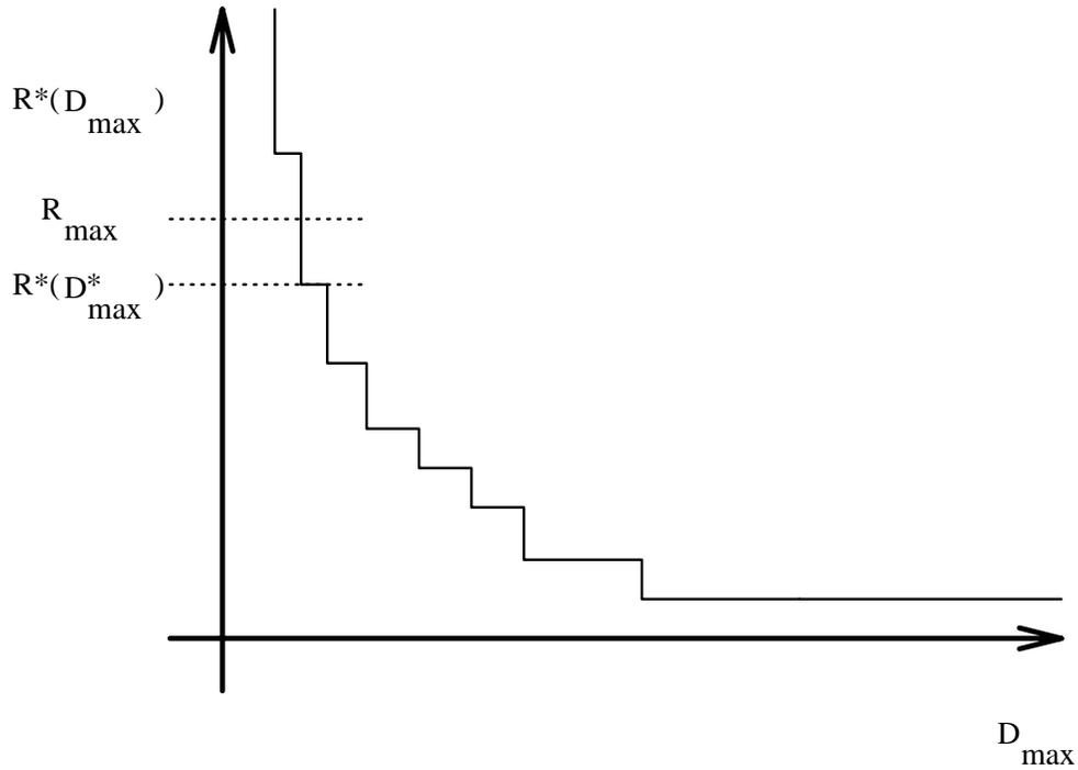
Figure 15: The  $R^*(D_{max})$  function, which is a non-increasing function exhibiting a staircase characteristic. The selected  $R_{max}$  falls onto a discontinuity and therefore the optimal solution is of the form  $R^*(D^*_{max}) < R_{max}$ , instead of  $R^*(D_{max}) = R_{max}$ .
