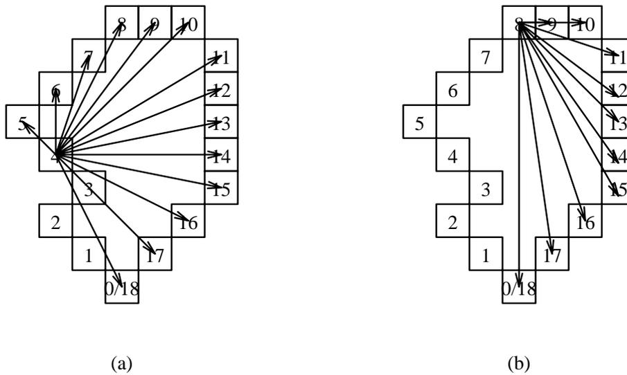
Figure 11: Interpretation of the boundary and the polygon approximation as a weighted directed acyclic graph. Note that the set of all edges  $E$  equals  $\{(a_i, a_j) \in A^2 : i < j\}$ . Two representative subsets are displayed: (a)  $\{(a_4, a_j) \in A^2 : \forall j > 4\}$  and (b)  $\{(a_8, a_j) \in A^2 : \forall j > 8\}$ .
