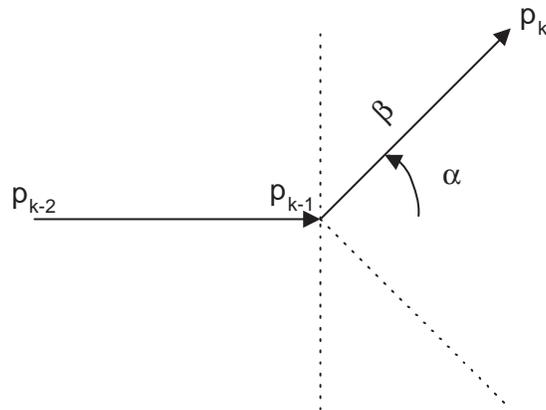
Figure 16: A simple second order DPCM scheme is used to encode the control points. The angle  $\alpha$  must take a value out of the following set:  $\{-90, -45, 45, 90\}$ . This is encoded with two bits. The length  $\beta$  is a number between 1 and 15 and is encoded using between 2 and 5 bits.
