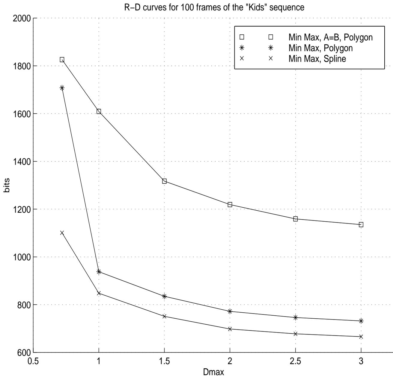
Figure 18: Average operational rate distortion curves for the first 100 frames of the "Kids" sequence.
