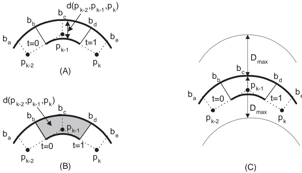
Figure 7: Three different ways for defining the segment distortion for a second order B-spline curve-based approximation of the original boundary. Figure (a) shows the maximum distance, Figure (b) the error area, and Figure (c) the maximum distance band concept.
