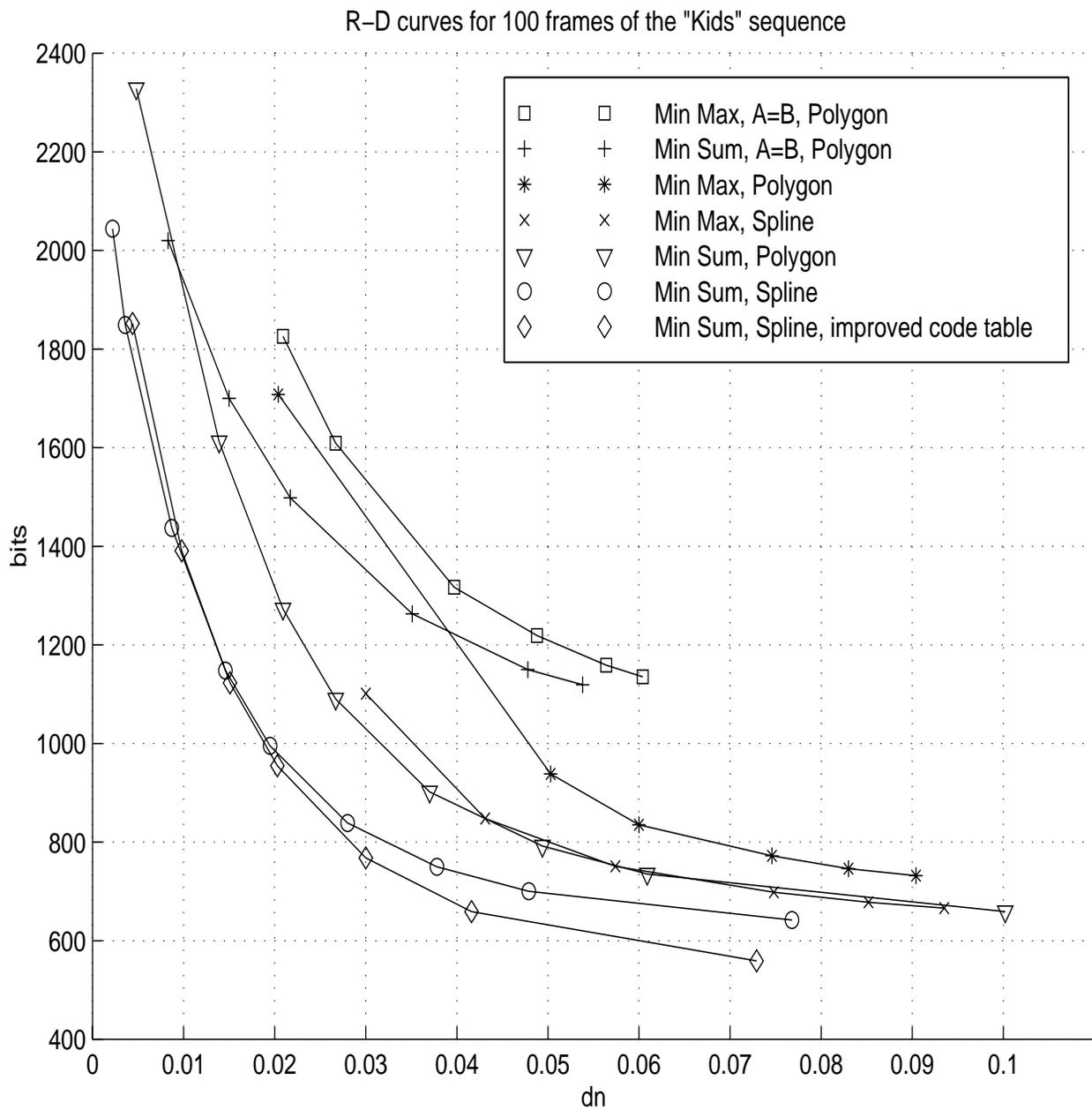
Figure 23: Average operational rate distortion curves for the first 100 frames of the "Kids" sequence.
