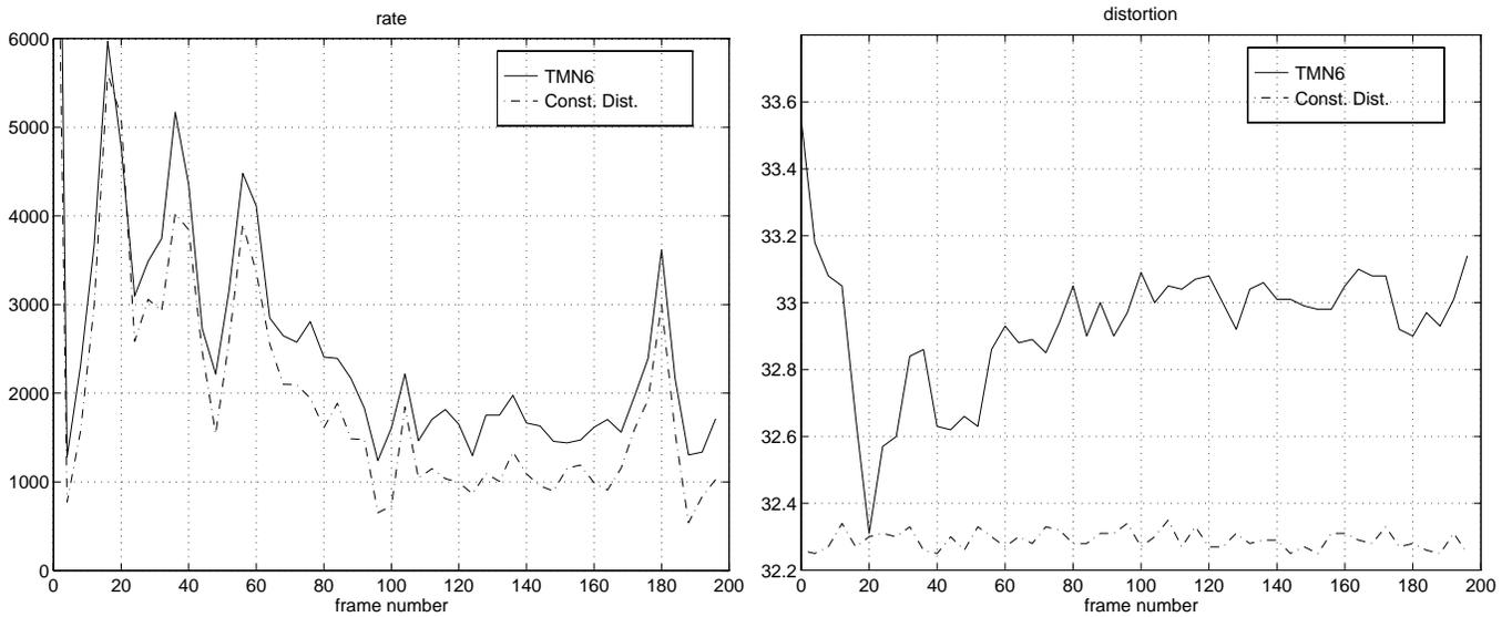
Figure 12: Rate and distortion comparison between TMN6 and the optimal coder, where the distortion of the optimal coder is fixed.
