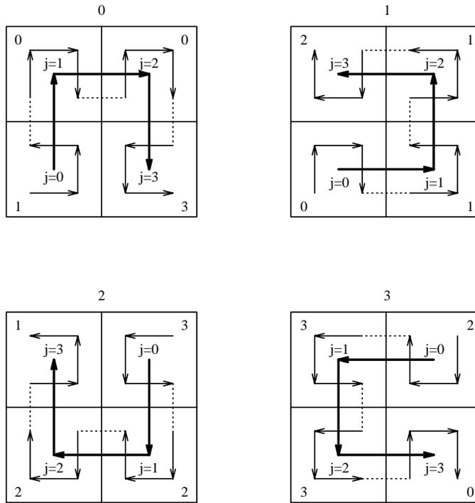
Figure 2: The four possible first order Hilbert curves (-) with the respective second order Hilbert curves underneath (-). The orientations  $O_{l,i}$  are shown on top of the squares and the orientations  $O_{l-1,4*i+j}$  are shown in the corners of the smaller squares.
