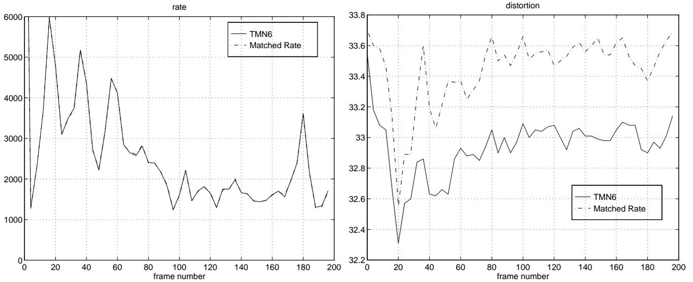
Figure 11: Rate and distortion comparison between TMN6 and the optimal coder, where the TMN6 rate is the target rate of the optimal coder.
