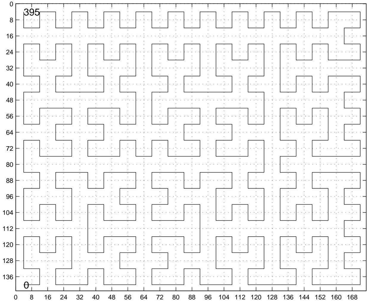
Figure 8: Modified Hilbert scan for level  $n_0 = 3$  of a QCIF frame.
