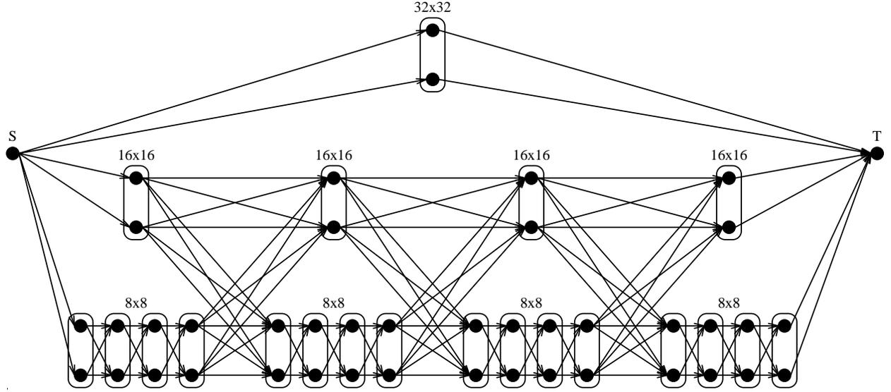
Figure 4: The multilevel trellis for  $N = 5$  and  $n_0 = 3$
