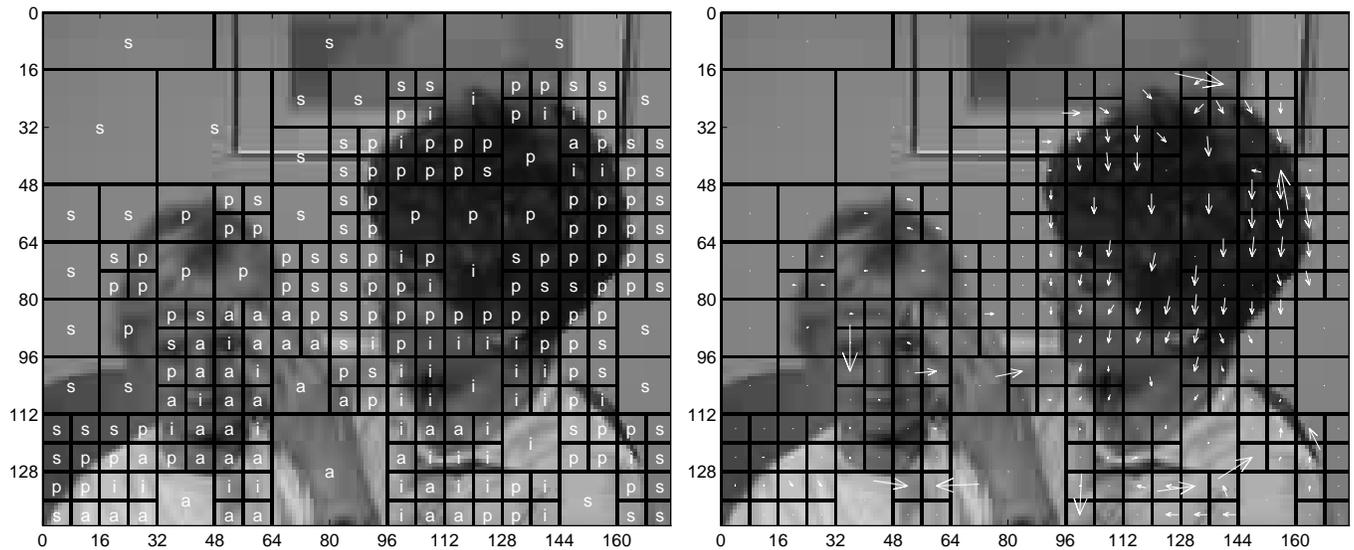
Figure 10: Left: The optimal encoding mode selection, (i) Inter mode, (s) Skip mode, (p) Prediction mode and (a) Intra mode; Right: the optimal DVF, both are for the 16<sup>th</sup> frame of the “Mother and Daughter” sequence.
