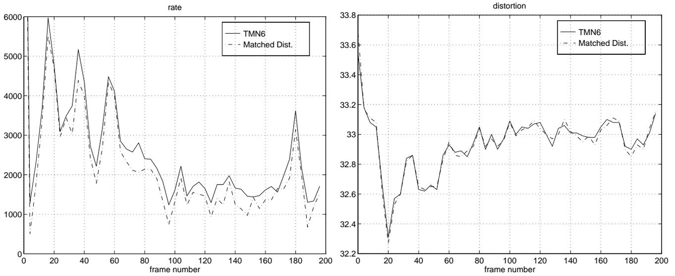
Figure 9: Rate and distortion comparison between TMN6 and the optimal coder, where the TMN6 distortion is the target distortion of the optimal coder.
