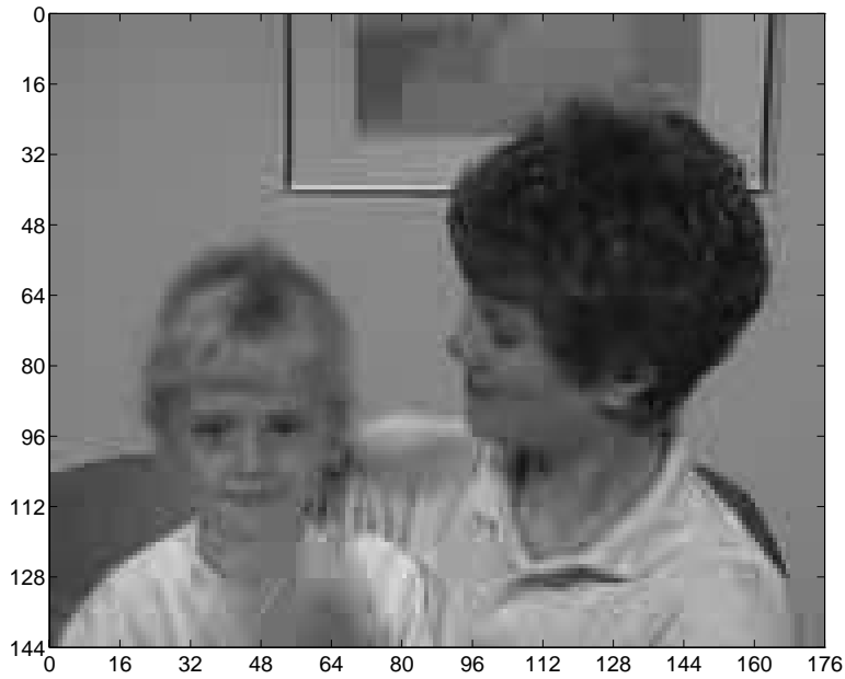
Figure 5: The 12 th reconstructed frame of the “Mother and Daughter” sequence. This frame is used to predict the 16 th frame.
