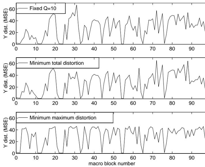
Figure 7: MSE of each macro block of the luminance channel; First row: MSE for a fixed quantizer step size of  $Q=10$ . Second row: MSE for the minimum total distortion approach. Third row: MSE for the minimum maximum distortion approach.
