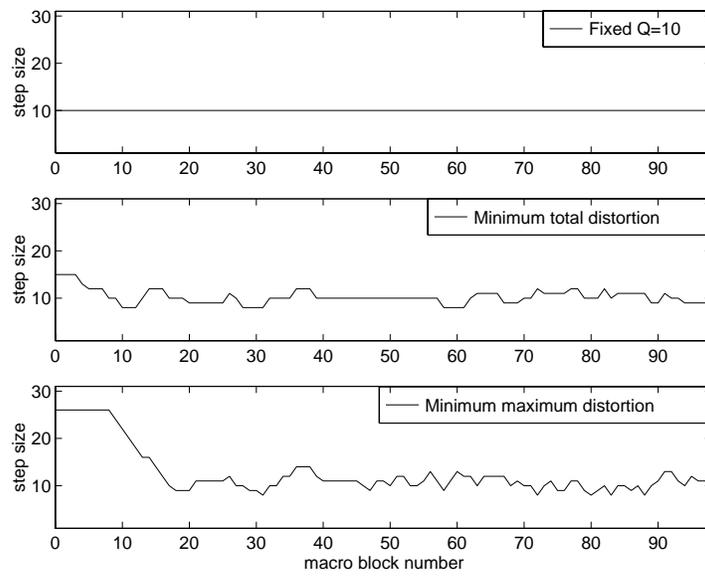
Figure 8: Macro block quantizer step sizes; First row: fixed quantizer step size of  $Q=10$ . Second row: step sizes for the minimum total distortion approach. Third row: step sizes for the minimum maximum distortion approach.
