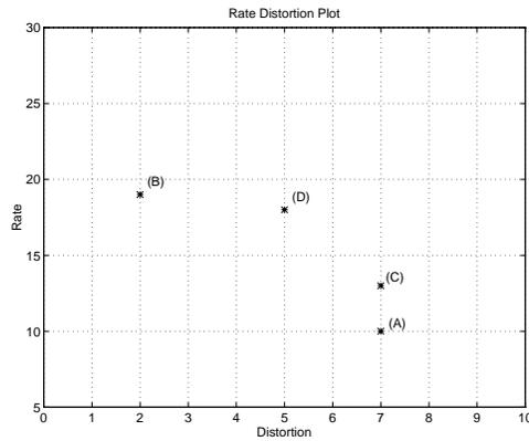
Figure 6: Operational rate distortion curve for the toy example, using the MIN-MAX criterion. Note that (C) is not part of the operational rate distortion curve, since (A) has the same distortion but a smaller rate. (C) is only included for completeness.
