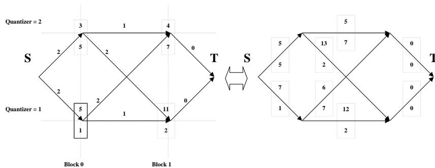
Figure 2: The graph (trellis) of the toy example. The left graph shows the rate required to switch the quantizer on top of the edges. The rate needed and distortion resulting by coding a certain block with a certain quantizer are displayed inside of the dashed boxes. The rate is above the node and the distortion below. The right graph is equivalent to the left graph, just that the all the rates and distortions are merged onto the edges.
