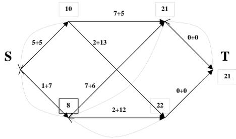
Figure 3: The graph for a  $\lambda$  of one. The dashed boxes contain the smallest Lagrangian cost up to and including the node. The dashed arrows are the backpointers used to remember the optimal
