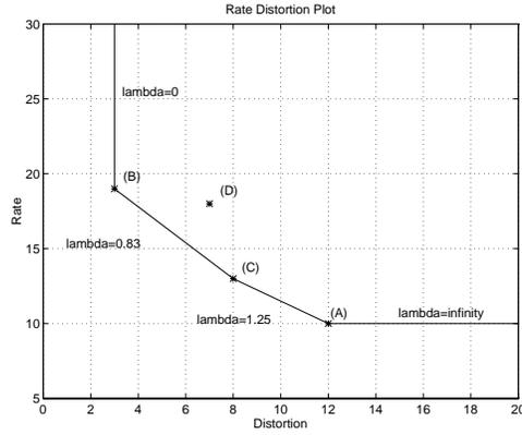
Figure 5: Operational rate distortion curve for the toy example, using the MI-NAVE criterion. Note the convex hull and the fact that the slope of the convex hull is related to  $\lambda$  as follows, slope =  $-1/\lambda$ .
