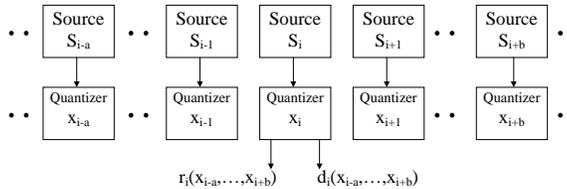
Figure 1: A dependent coding framework: the source rate and distortion depend on a neighborhood of quantizers
