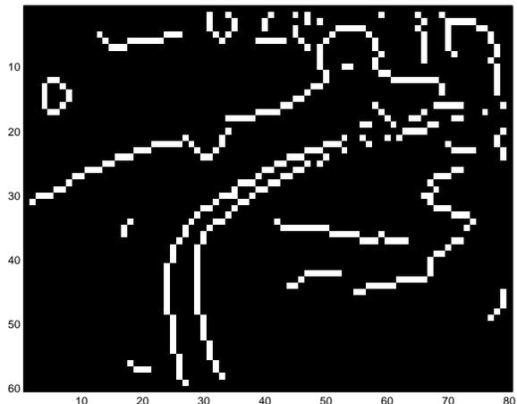
Fig. 3. Canny edge detector processing the image shown in fig. 1
