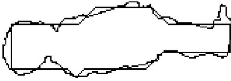
**Figure 3: Shape approximation with the base layer only (R=73 bits, D=917 pels).**
