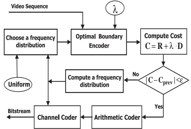
Figure 4: The entropy encoder structure.
