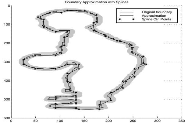
Figure 1: Admissible control point band.
