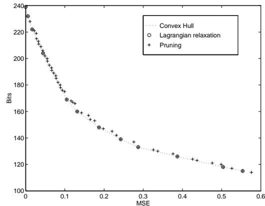
Figure 3. Operational rate distortion curve
