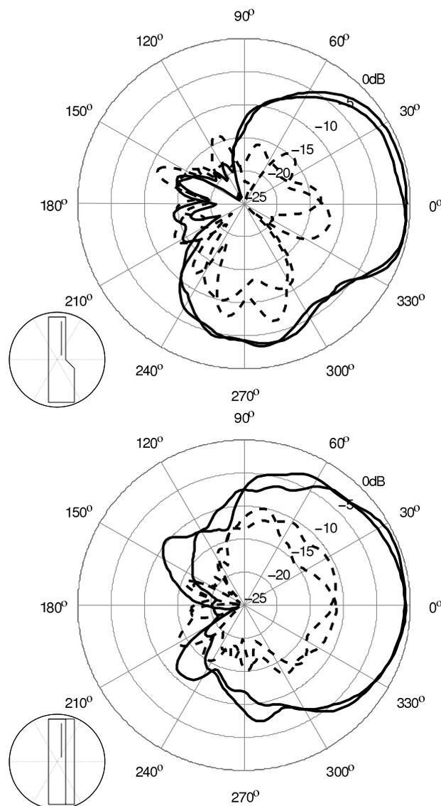
Fig. 6. Vertical (top) and horizontal (bottom) antenna pattern of two antenna prototypes with different spacing at 5.8 GHz. Solid: LHCP, dashed: RHCP.
