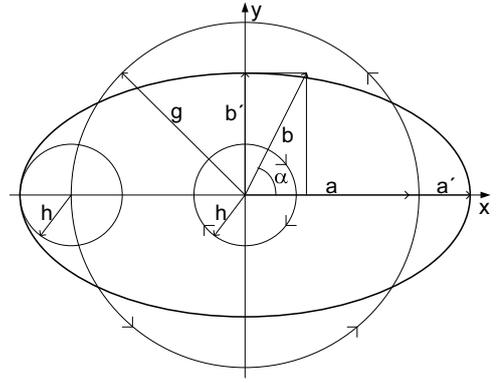
Fig. 3. Axial ratio and cross-polarization calculation.
