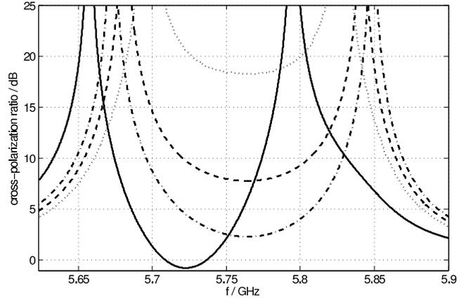
Fig. 4. Calculated PR depending on frequency and power distribution between both modes. Dashed:  $a/b = 0\ \text{dB}$ , dash-dotted:  $a/b = -2\ \text{dB}$ , dotted:  $a/b = +2\ \text{dB}$ , solid:  $a/b$  depends on  $\Gamma_i$ .
