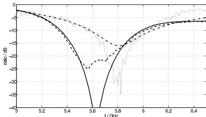
Fig. 5. Return-loss and polarization of an antenna prototype with spacing of 3.5 mm between case and PCB. Solid: simulated  $|S_{11}|$ , dashed: measured  $|S_{11}|$ , dash-dotted: simulated CPR, dotted: measured CPR.
