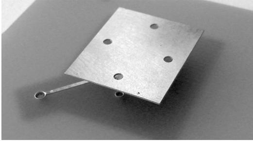
Fig. 2. 5.8 GHz microstrip antenna on FR-4 substrate without case.
